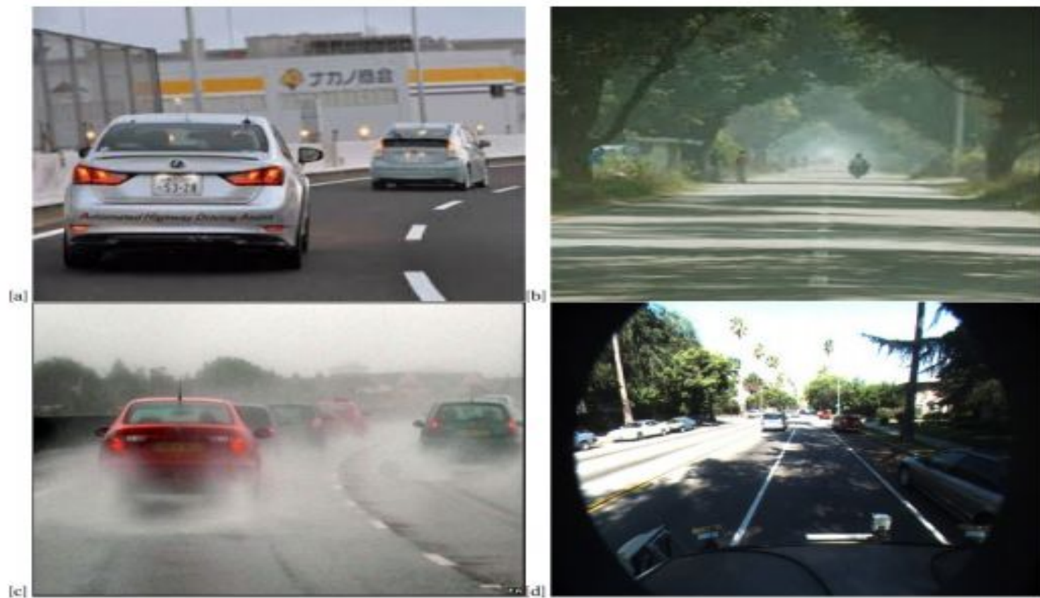
Figure. 2 Various challenges in lane detection.[a] A vehicle occluding nearby lane [b] Presence of shadow[c] Rainy road [d] Extreme illumination on left side of image
